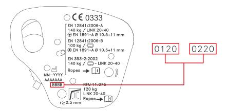
Anyone in possession of a device marked with one of these two batch numbers must immediately stop using the device and carry out the test described here below.
