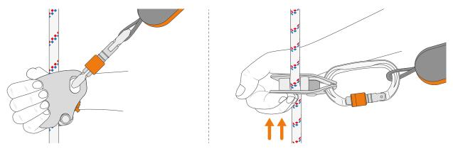
In the picture, the user grabs the openable side plate squeezing it towards the locking cam. This pressure, even after removing the hand from the device, could lead to a delay in the locking onto the rope in the event of a fall.
